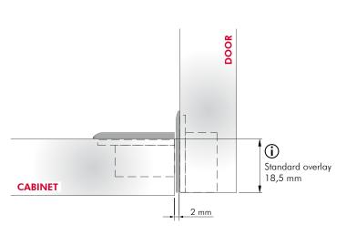
The overlay value can be reduced by adding bespoke adapters on the cabinet side.
