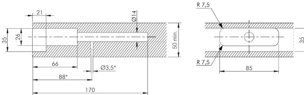
\* Optional drilling for security locking with M4 grub screw placed underneath in alignment with the cavity. For details refer to Triade Pro Maxi section.
