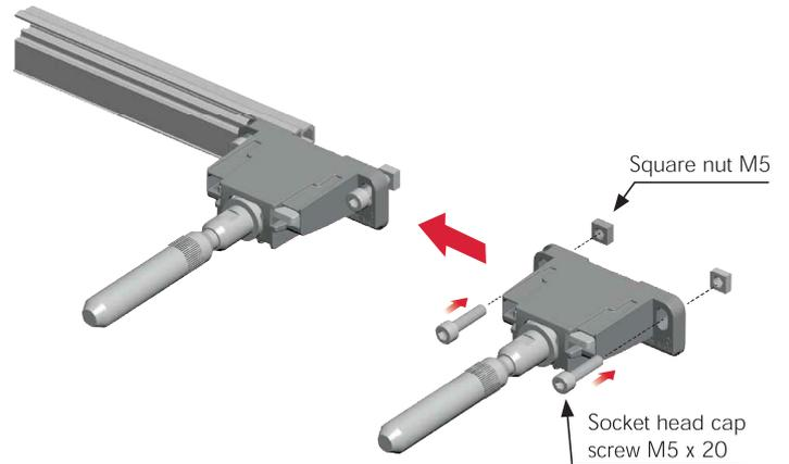
INSTALLATION ON THE WALL AND SHELF INSERTING
