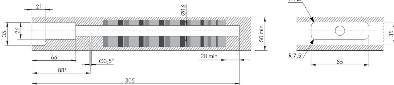
\* Optional drilling for security locking with M4 grub screw placed underneath in alignment with the cavity. For details refer to Triade Pro XXL section.
