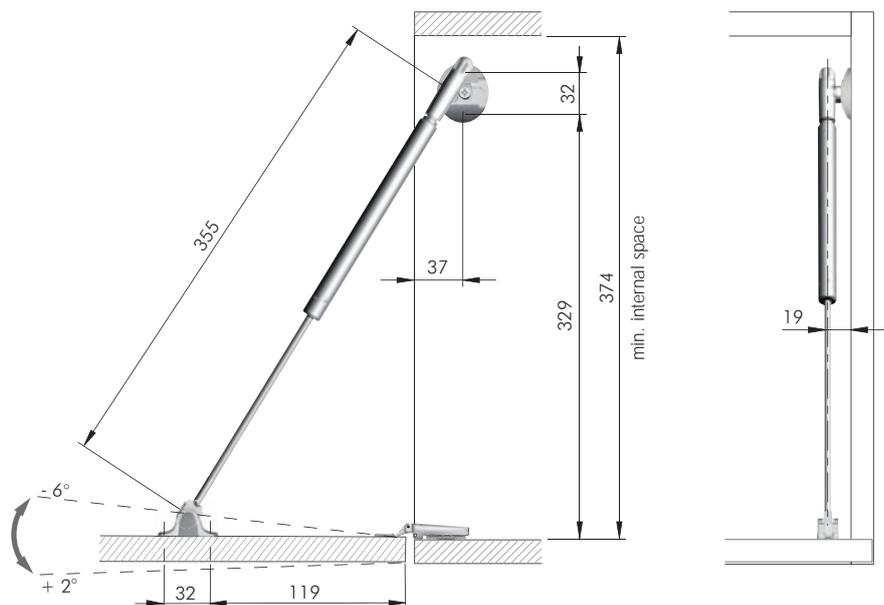
The dimensions of the drilling plans refer to carcasses which use **standard sprung hinges** and mounting plates 0 mm. Please note that the opening angle shown data is purely indicative. It varies with respect to the hinge brand and adjustment carried out.
