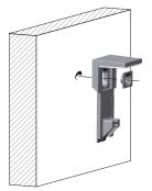
Recommended fixing countersunk screw type - head  $\emptyset$  5 mm max.
