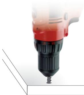
3 - Screw the assembly fitting into the face bored panel using a cross screwdriver.
