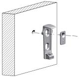
Recommended fixing countersunk screw type - head  $\varnothing$  4 mm max.
